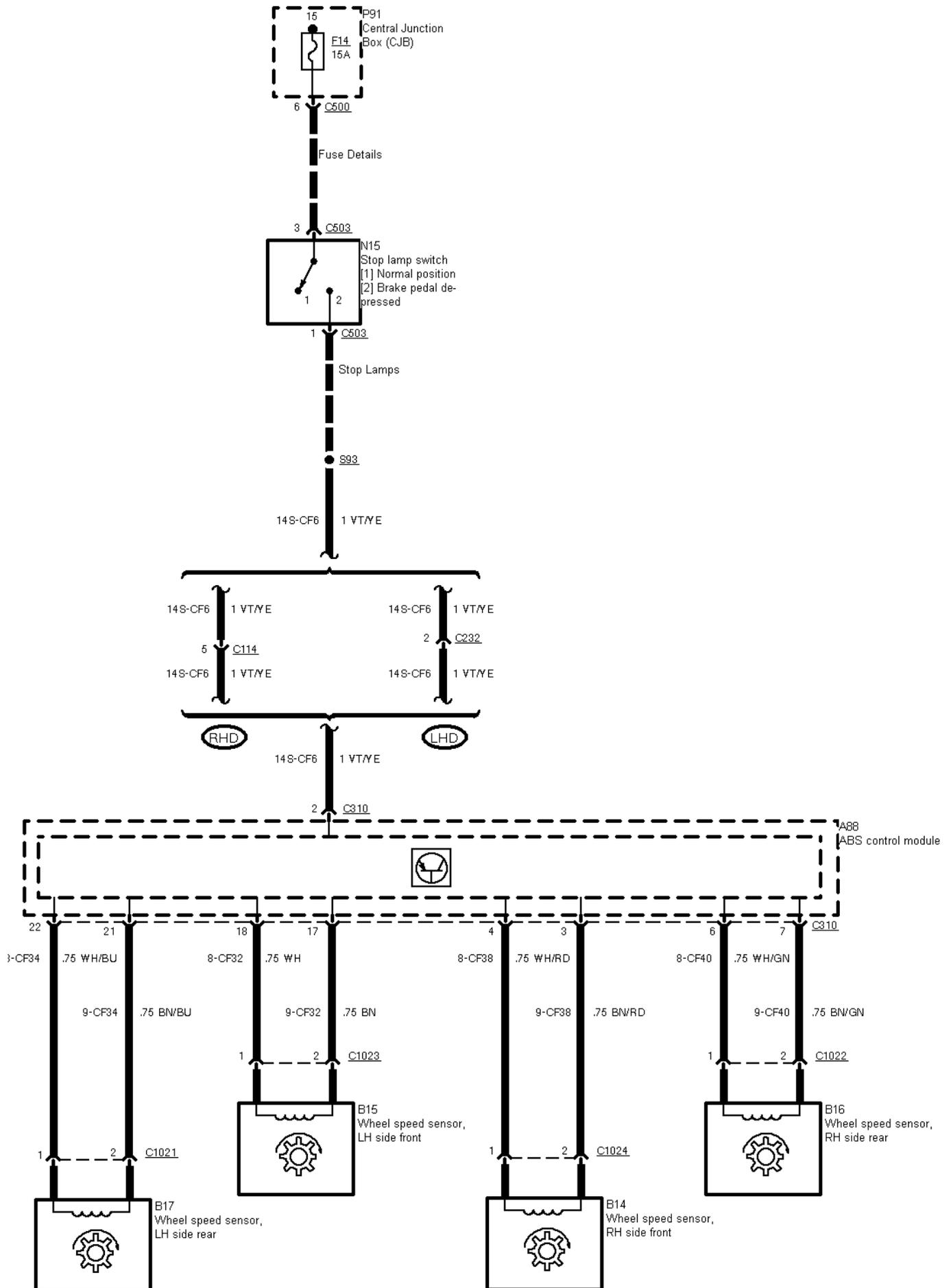
12-03-003 , Anti-lock Braking System (ABS) MK 20-I , Diagnostic connectors
