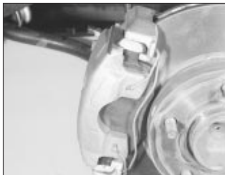
7.2 Spring clip fitted to outboard face of front caliper
