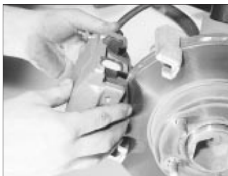
7.5 Lifting a front caliper off the disc
