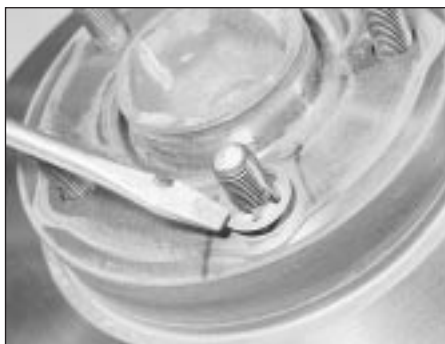
5.3 Disc-securing spring clip
