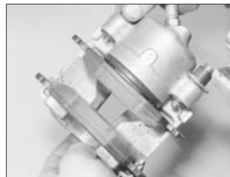
7.8b Both pads fitted to a front caliper
