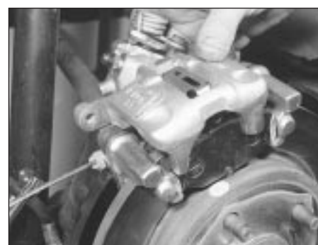
11.5b . . . and remove the rear caliper
