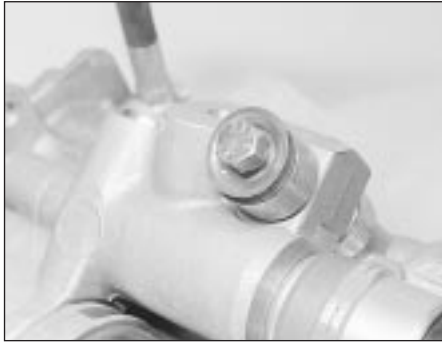
18.5 Hydraulic unit pump mounting bolt
