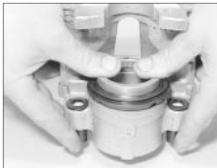
10.9 Pressing the piston into the bore
