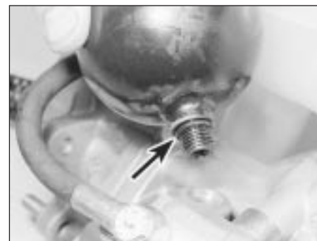
17.4 Removing the accumulator Note O-ring (arrowed)
