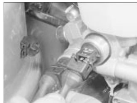
15.3c Disconnecting the main valve plug
