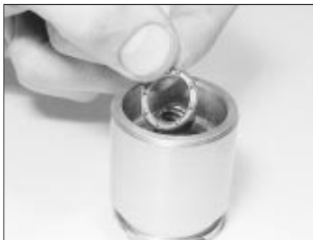
12.4d . . . the thrust bearing . . .
