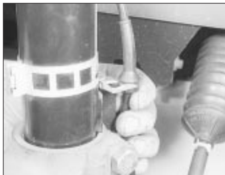
26.4 Unclipping the sensor wire from the strut
