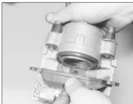
7.8a Clipping the inboard front pad into the piston
