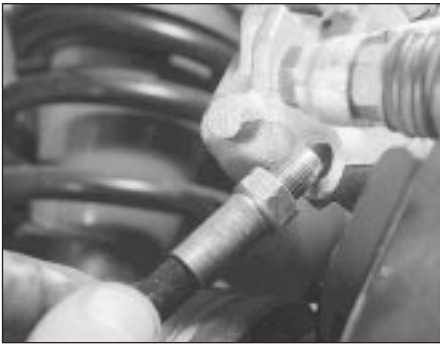
21.5 Disconnecting the hose from the caliper
