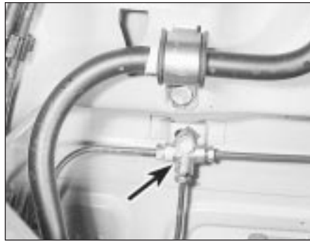
21.7 Brake pipe union T-piece (arrowed)
