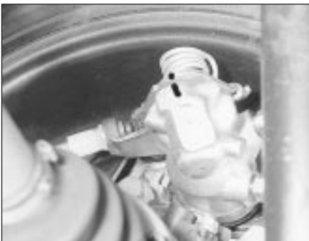
22.4 Alignment marks painted on lever and body
