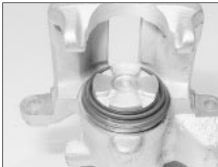
12.21 Dust boot fitted to caliper and piston
