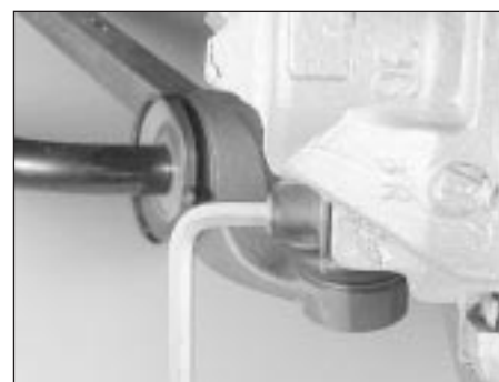
7.4 Undoing a caliper slide bolt
