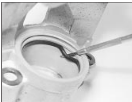
10.5 Removing the piston seal
