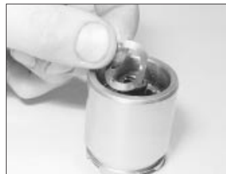
12.4c . . . a wave washer and (not shown) another thrustwasher . . .
