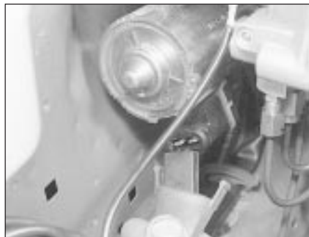
15.3e Disconnecting the pump motor plug
