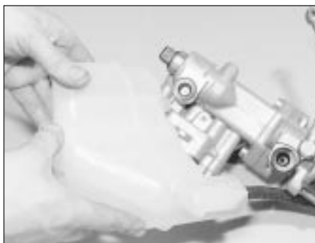
16.6 Removing the hydraulic fluid reservoir
